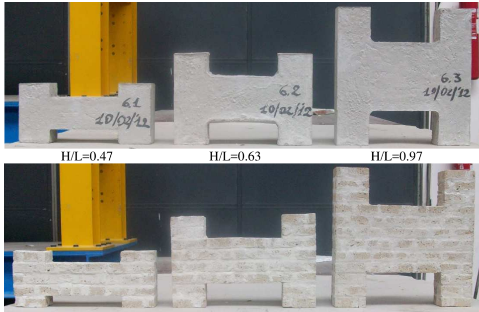
Fig. 2b - H-shaped specimens in homogeneous materials and ordinary masonry
