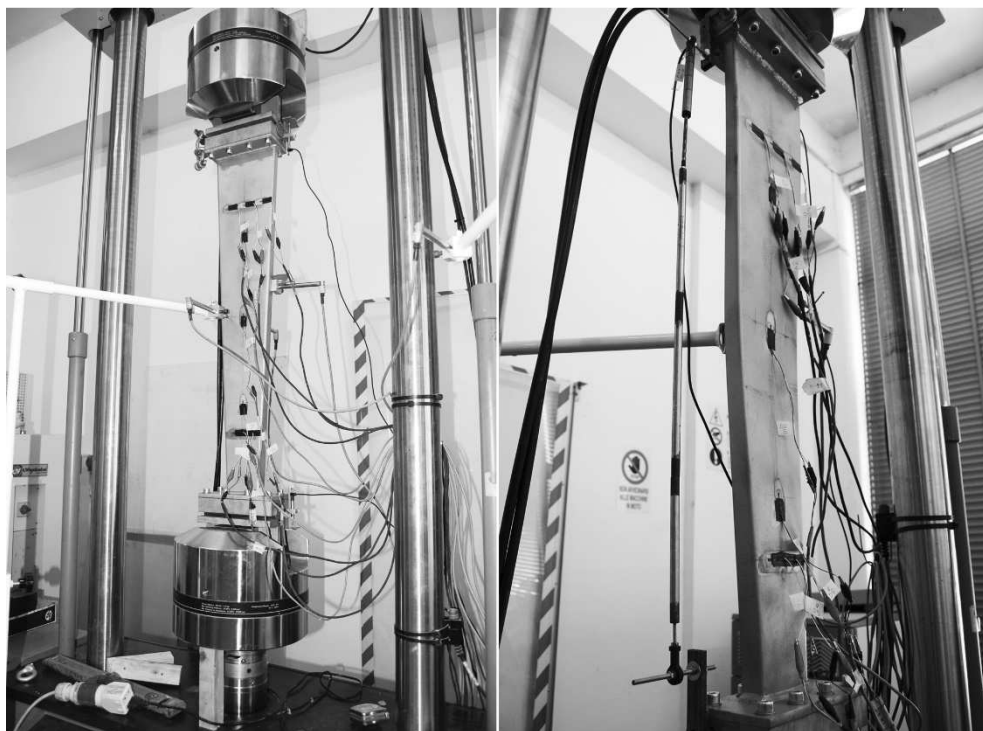
Fig. 3 – Tested beam: pre and post buckling
